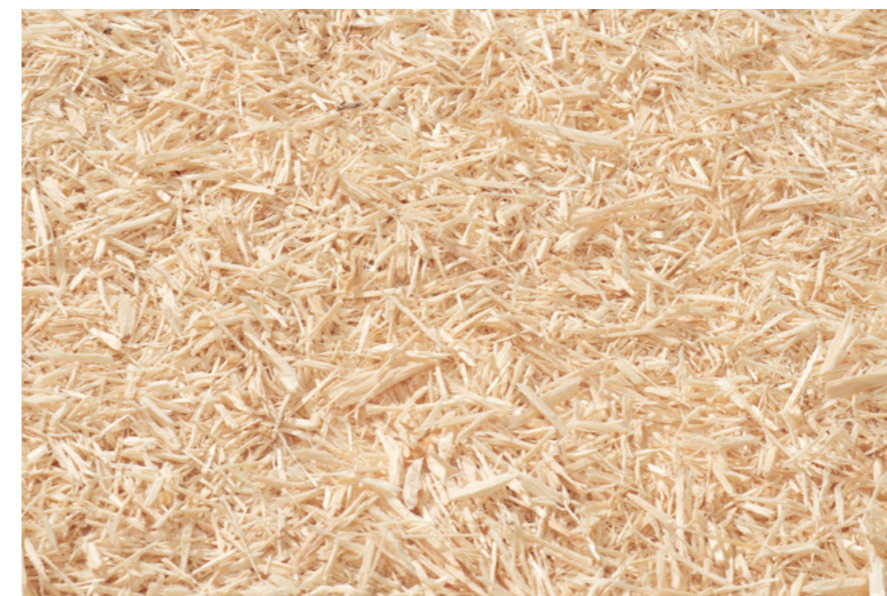
↑ Wood chips downstream of the hammer mill
