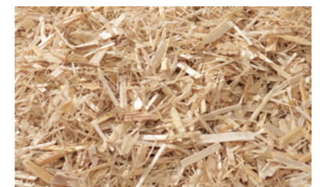
↑ Safflower straw downstream of the hammer mill
